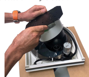
Figure 12 - Lowering camera assembly onto the standoffs.
