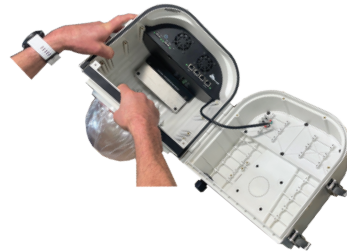
Figure 2 - Removing the lower tray assembly.
