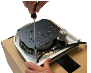
Figure 13 - Securing camera mount assembly to the standoffs.
