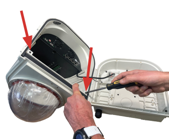
Figure 1 - Removing lower tray fastening screws.
