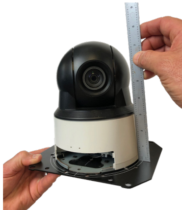
Figure 8 - Measuring the height of camera assembly.
