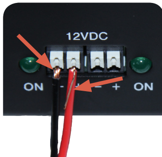
Figure 1.6.1 - Exposed Wire & Poor Connection
